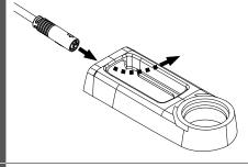
Feed the connecting cable for the display / Smart Box cleanly through the display enclosure in the frame.
