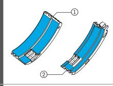
Apply the pre-cut gap pads onto the cooling fins.
