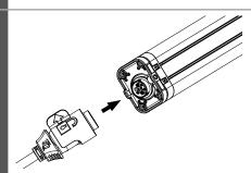
Connect the battery plug from the wiring harness to the battery.
