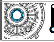
Mount both cranks with appropriate grease and according to crank manufactueres tightening torque.
