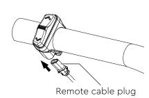
Insert the oval plug of the remote cable properly aligned and all the way into the remote control unit. Feed the cable within the handlebars in the direction of the display.
