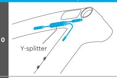
Y-splitter installed and connected between display and harness.
