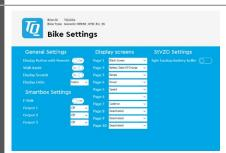
Under the menu item "Bike Settings", the required outputs for the electronic circuitry or the lighting can now be enabled.
