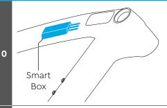
Smart Box installed and connected between the display and the wiring harness.
