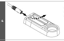
Feed the connecting cable for the display / Smart Box cleanly through the display enclosure in the frame.
