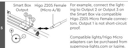
For example, connect the lighting to Output 2 or Output 3 on the Smart Box via compatible Higo Z205 Micro Female connectors. Output 1 is not short-circuit proof.
