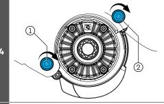
Tighten the motor bolts ① and ② according to the respective e-bike manufacturer with a tightening torque of 20 Nm. Use new motor bolts (using a medium-strength threadlocker if necessary)
