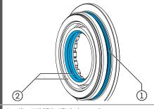
Prior to assembly of the lockring, grease the O ring ①
