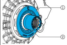
Place the chain ring (manufacturer-dependent) on the output shaft.
