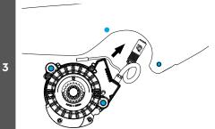
Insert the drive unit into the e-bike frame – matching the mounting points.
