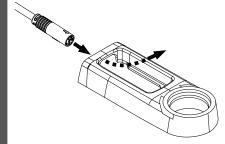
Feed the connection cable for the display / Y-splitter cleanly through the display pocket in the frame.
