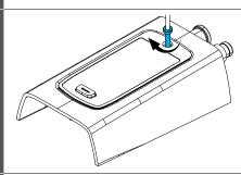
Tighten the included M3×20 display screw with a torque of 0.5 Nm.
