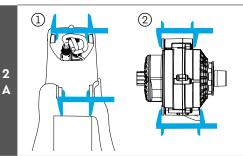
① Use a caliper gauge to measure the distance between the two mounting points in the frame.
