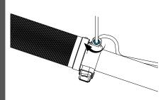
Tighten the pre-assembled M3 remote screw using a torque of 1 Nm.
