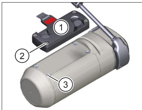
Fig. 3: Fasten FIDLOCK® Force Connector to Range Extender
