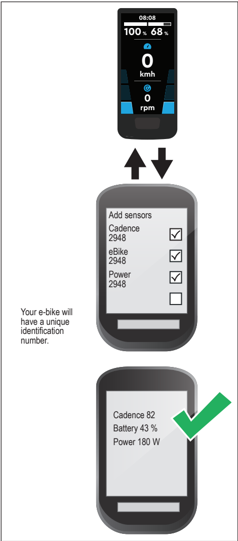
Fig. 8: Connection e-bike to bicycle computer
